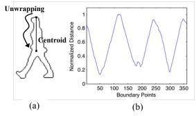
Fig. 3. Silhouette representation: (a) Boundary extraction (b) Distance between the centroid and each border pixel [3]
