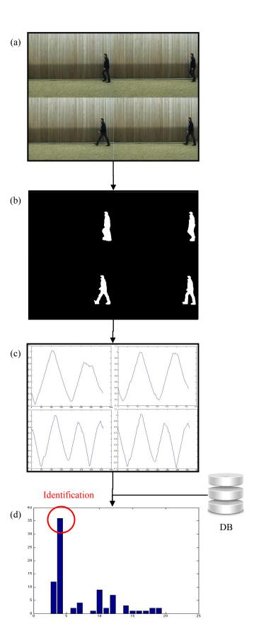
Fig. 5 Identification process: (a) 4 frames of a test sequence. (b) Respective extracted silhouettes for the 4 frames. (c) Distance signal corresponding to the silhouettes. (d) Histogram representing the number of silhouette found in the test sequence for each person.
